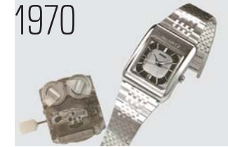
QUARTZ ASTRON 36SQC, the world's first watch to integrate a CMOS IC
