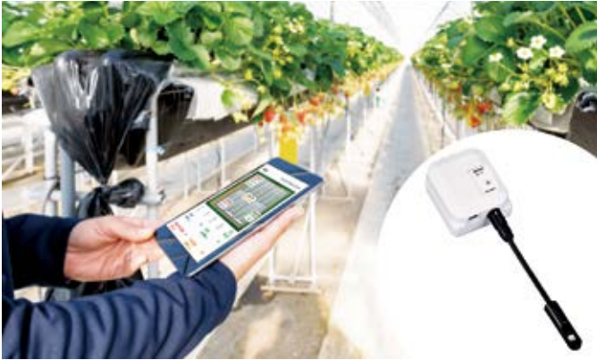
Wireless temperature and humidity sensors (right) are battery powered, can be installed anywhere, and offer monitoring of every corner with the placement of multiple sensors throughout the greenhouse
