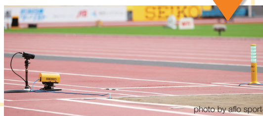
photo by aflo sport If the lamp is green, the attempt is successful. If red, it is a foul.
