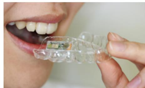
Wireless sensor module mounted on a mouthpiece
