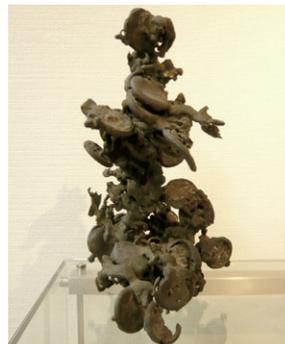
Pocket watches sent in for repair that were destroyed by fire due to the Great Kanto Earthquake of 1923
