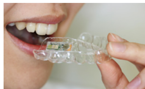
Wireless sensor module mounted on a mouthpiece
