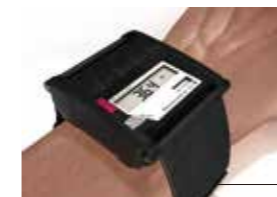
Watch-type vital sensor for applications such as managing heat stroke risk at construction sites
